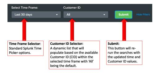
The Customer ID is populated by a search run within the selected time frame. If a new time frame is selected the Customer ID options will dynamically update. In order to apply a new time frame or select a specific Customer ID the 'Submit' button must be selected.
